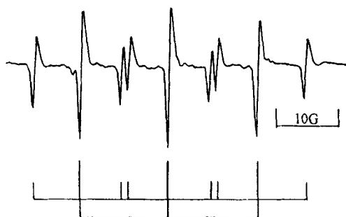
FIG. 4. EPR spectrum of BDCA/MNP system obtained after irradiation at room temperature: 1 \text{ mT} = 10 \text{ G} , [\text{BDCA}] = 0.20 \text{ mol} \cdot \text{L}^{-1} , [\text{MNP}] = 0.022 \text{ mol} \cdot \text{L}^{-1} .
